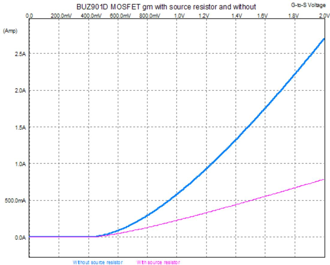
The formula for the decrease in a MOSFET's gm because of an unbypassed source resistor is:
