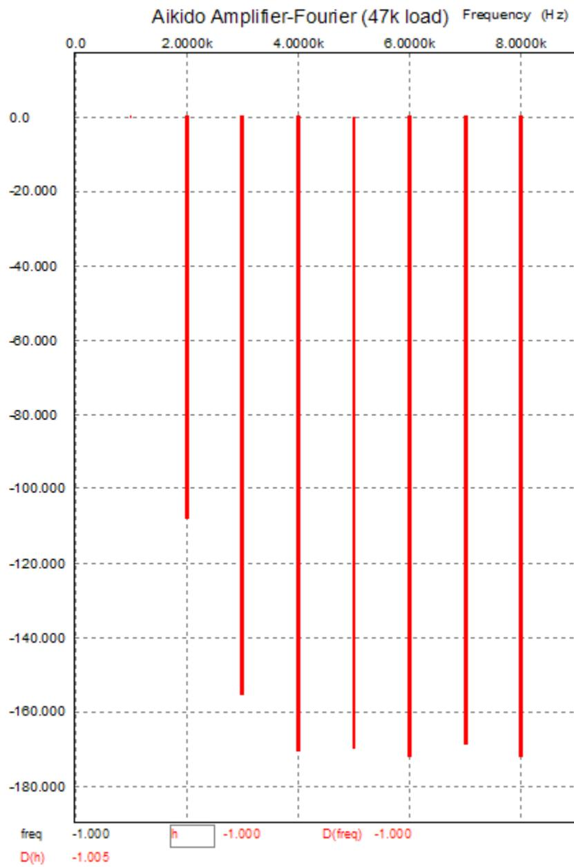
The winner is obvious in terms of distortion; both tie in output impedance; and the Aikido (using all 6922s) only has a gain of 16 (+24 dB). What if we swapped some of the current-mirror-based amplifier's gain for linearity?
