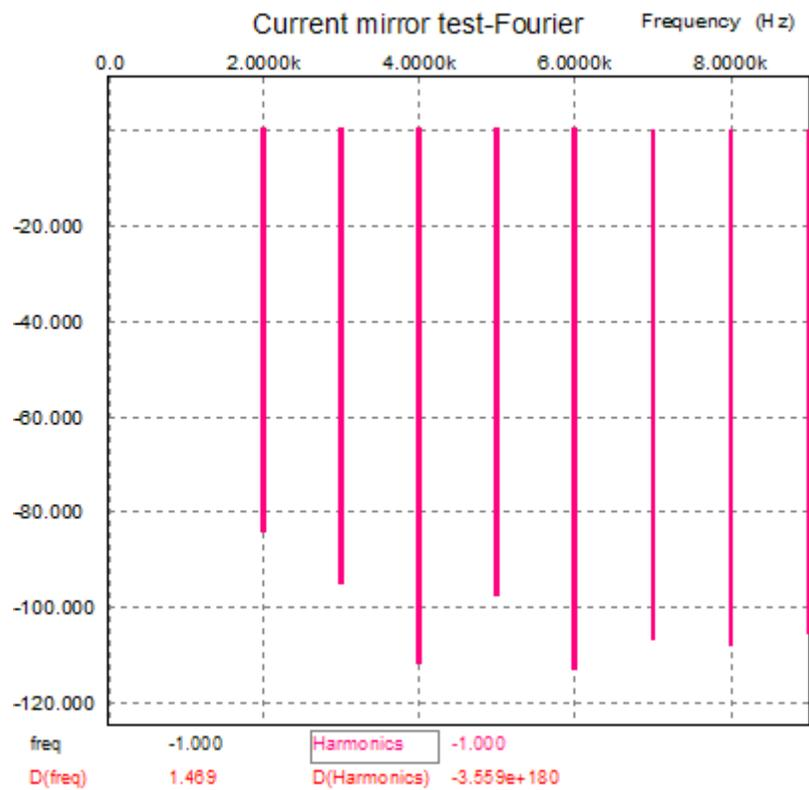
When using a transistor-based current mirror, I always match the transistors, believing it critical, besides my VOM holds a hfe test, which makes the matching painless. Well, using unmatched transistors, with one having twice the beta as the other, only slightly increased the distortion and reduced the current mirroring efficiency by less than one percent, so maybe I have been overly nervous.
