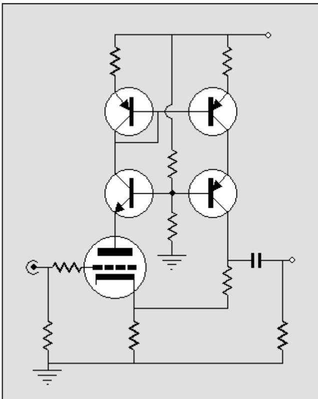
Still, the problem this topology faces is that it does not improve upon a grounded-cathode amplifier's PSRR. Inverting the cascode and adding a constant-current source will take care of the PSRR troubles, as the B+ noise cannot make across the constant-current source.
