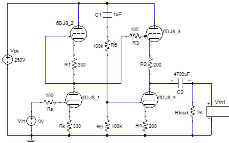
Above is a schematic of the circuit used in the **B<sup>2</sup> Spice A/D simulator**. The idle currents were close with 8.22mA for the first stage and 11.88mA for the second stage.
