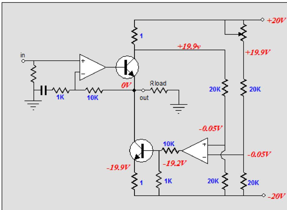
How does the amplifier work? Basically, it the White cathode follower (Taylor circuit) all over again. The flow of current through the top output device controls the flow of current through the bottom output device. When the input signal
