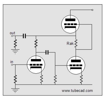
Here's a test: Find the feedback loop in the above schematic. The answer is that the input tube's plate resistor defines a feedback loop, as it brings the SRPP's output back in inverted form to the bottom triode's grid (input).
