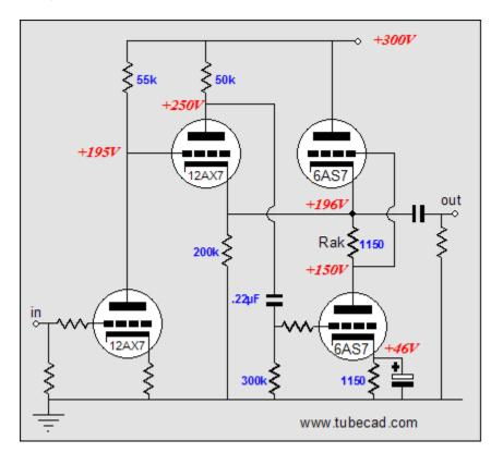
**Putting it all together** Combining the supercharged top and bottom half results in the circuits below:
