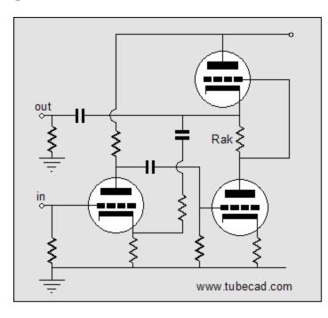
The above schematic shows an alternative approach. The input tube's plate resistor now terminates into the B+ connection and the added feedback-loop resistor returns to its cathode. Nothing fancy is going on here, as the input triode and the bottom output tube define a generic cascaded two-tube grounded-cathode amplifier that includes a feedback loop, as shown below.
