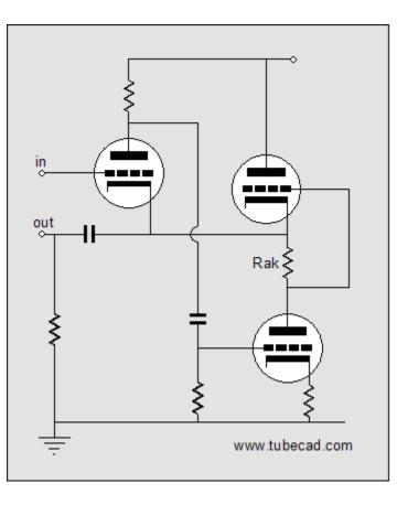
Which version is better? Better for what? is my usual reply. If the circuit is going to be a standalone buffer, then the first approach offers a ground-level input. If the buffer is going to be part of a larger circuit and it receives its input signal at some higher-than-ground voltage, the second approach will do away with the otherwise-needed coupling capacitor. For example:
