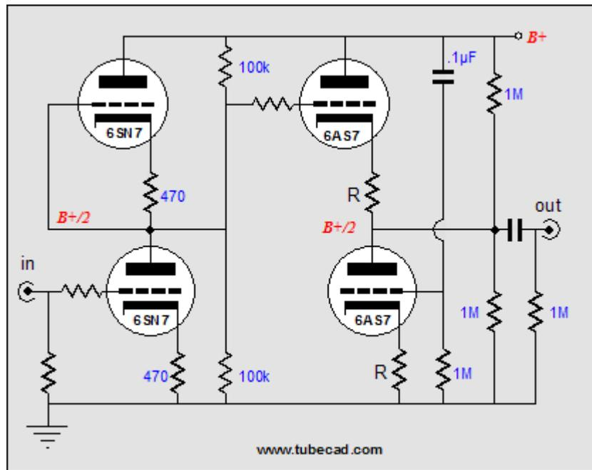
Notice the missing voltage divider; all of the power supply is presented to the bottom triode's grid.
